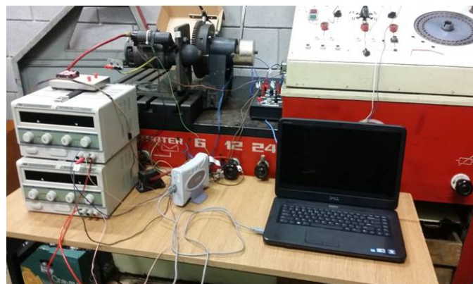
Figure 10. View of the measurement stand for testing the starter with the Hall sensor.
